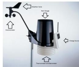
Image 1: This is an image from the website for the Vantage Pro2 Weather Station to which we have added identifiers. This shows what our barometer, weather vane, anemometer, rain gauge and thermometer look like.
